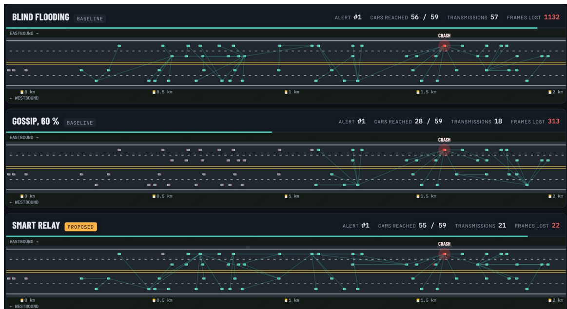
Figure 9.5: The whole 2 km road 30 ms after the crash. Lines show which car each vehicle received the alert from
